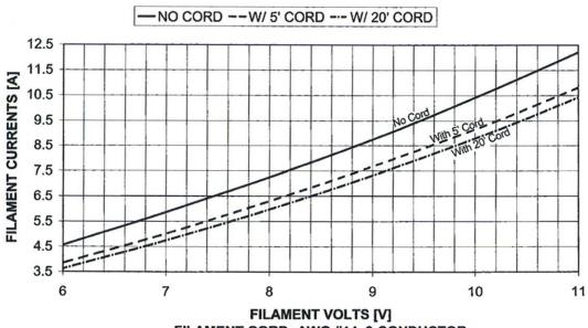
FILAMENT CORD: AWG #14, 2-CONDUCTOR
